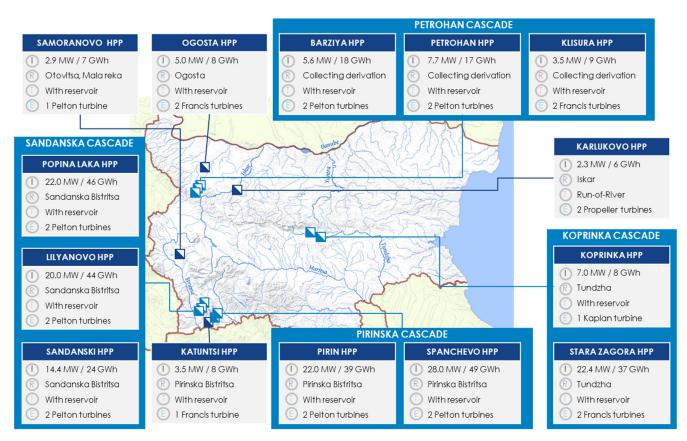
Legend: I – installed capacity and 2019 annual generation; R – river; T – type of the HPP (with reservoir or runof-river); E – # of turbines + type
