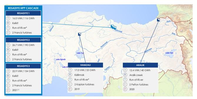
Legend: I – installed capacity and 2019 annual generation; R – river; T – type of the HPP (with reservoir or runof-the-river); E – # of turbines + type; F – end of FiT period (for Resadiye it applies to all HPPs in Resadiye cascade) EPAS Group estimates the long-term average electricity generation of its Turkish HPPs to amount to approximately 558 GWh.
