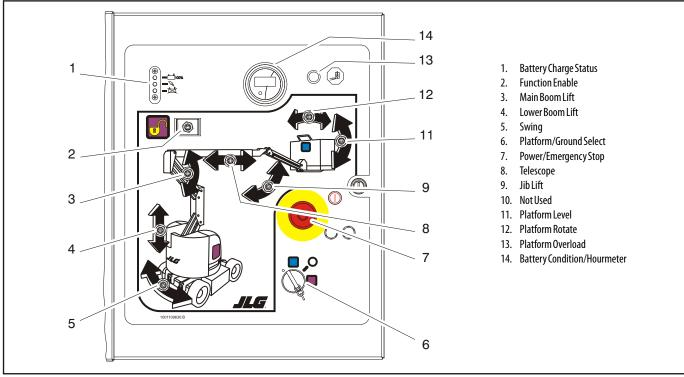
Figure 3-1. Ground Control Station - E300AJ
