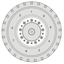
**3.** The tightening of the nuts should be done in stages. Following the recommended sequence, tighten nuts per wheel torque.
