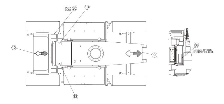
Figure 4-10. Decal Location Sheet 5 of 5
