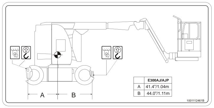
Figure 4-5. Lifting and Tie Down Chart
