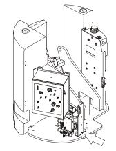
Lube Point(s) - Remote Fitting Capacity - A/R Lube - BG Interval - Every 3 months or 150 hrs of operation Comments - Apply grease and rotate in 90 degree intervals until bearing is completely lubricated 2. Swing Bearing/Worm Gear Teeth
