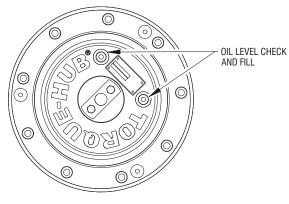
Lube Point(s) - Level/Fill Plug Capacity - 25.5 oz. (0.75 L)(1/2 Full) Lube - EPGL Interval - Check level every 3 months or 150 hrs of operation; change every 2 years or 1200 hours of operation 6. Wheel Bearings
