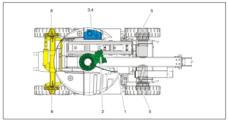
Figure 6-1. Operator Maintenance and Lubrication Diagram
