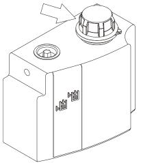
Lube Point(s) - Fill Cap Capacity - 2.9 Gal. (11 L), 2.1 Gal. ( 8 L) to Full Mark Lube - HO
