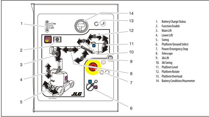
Figure 3-3. Ground Control Station - E300AJP
