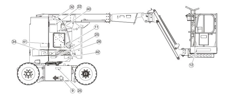
Figure 4-8. Decal Location Sheet 3 of 5
