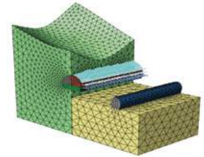
Steel pipe reinforced grouting (Pipe Roof) ▲
