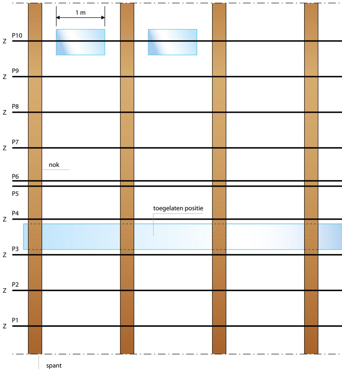
If the skylights are located perpendicular to the purlins, a width of 1 m is allowed. The roof ensures that the purlins stay in place in case of skylights between two adjacent roof purlins.
