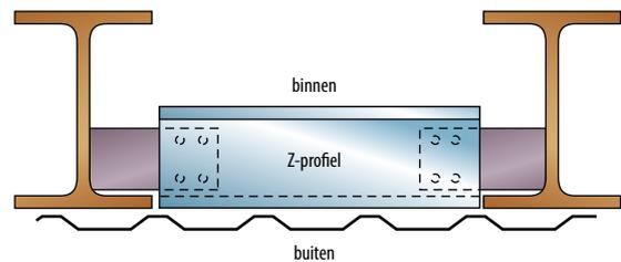
Figure C side rails between the rafters
