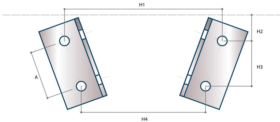
The cleats must be mounted to the steel structure. The Delta profiles must be placed and mounted in the cleats. Use bolts M12x30 (Delta 120-140-160-180-200-220) and bolts M16x30 (Delta 250-300). The installer must ensure that the top of the Delta purlin is level with the top of the girders.
