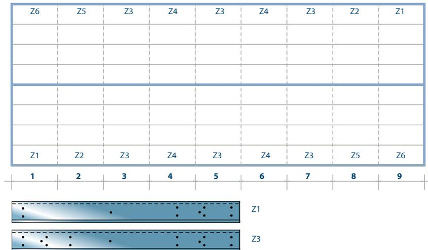
Above bays 1 and 3, the purlins are mounted with the small flange (B2) facing upwards through the additional mounting hole. The purlin can be fully secured at the end wall.
