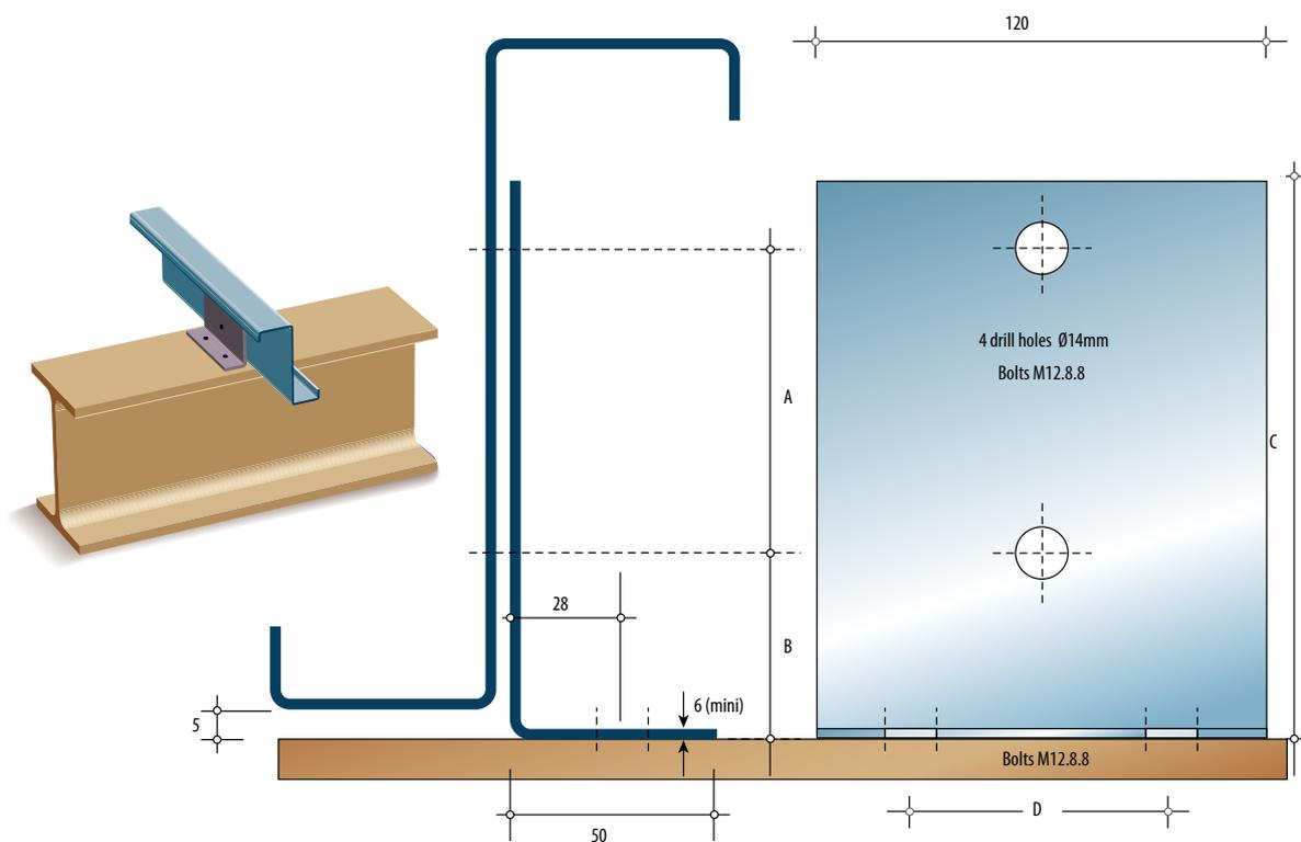
Type 2: The same system is used if the side rail is mounted to the columns.
