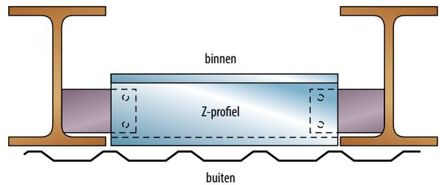
Figure C - side rails between the rafters
