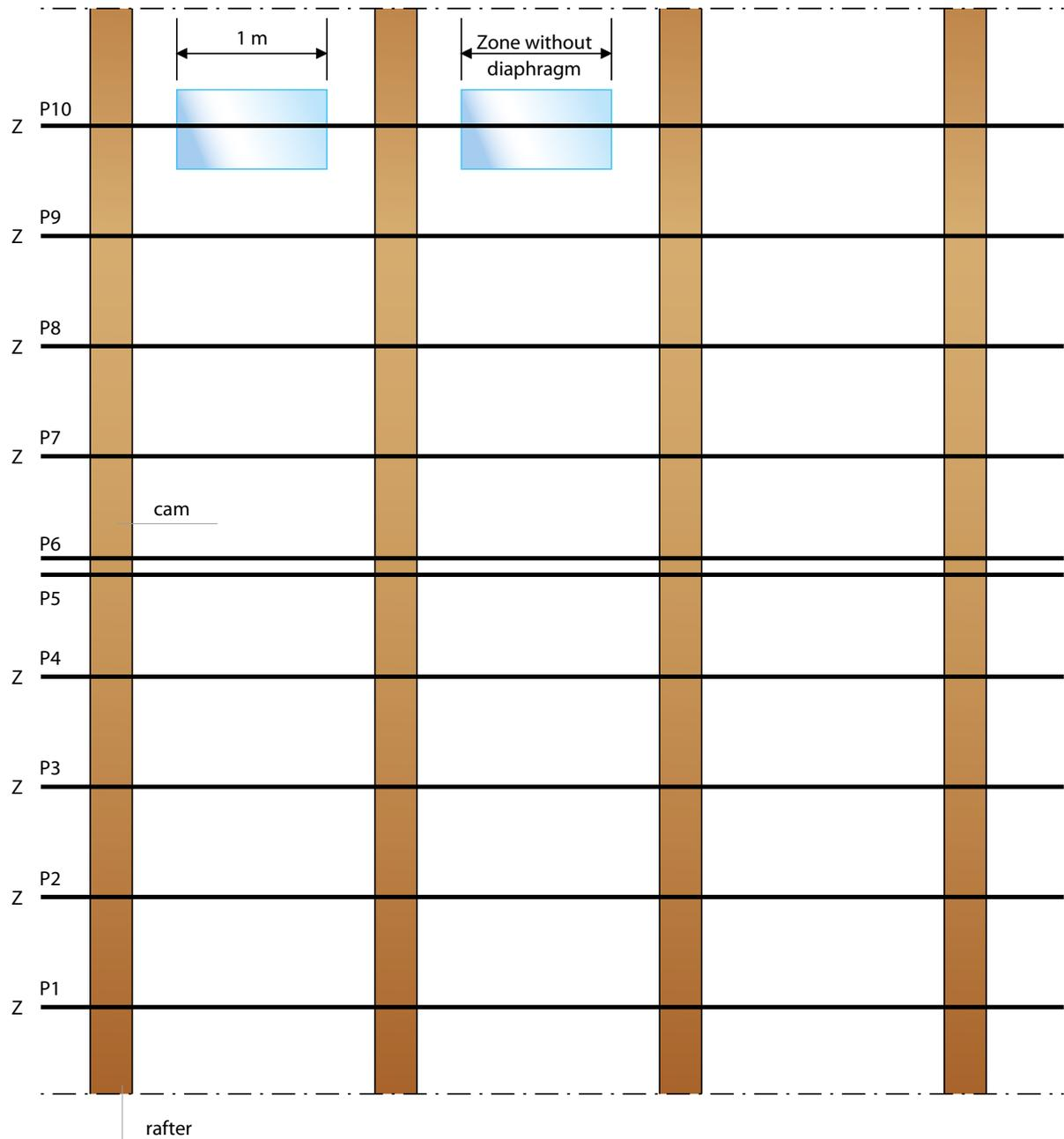
If the skylights are located perpendicular to the purlins, a width of 1 m is allowed. The roof ensures that the purlins stay in place in case of skylights between two adjacent roof purlins.
