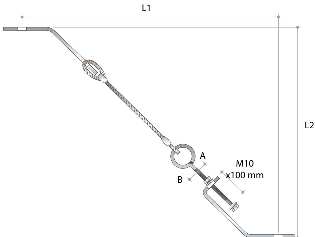
Cleat end perforation  $\varnothing 14 \text{ mm}$  (Z140 to Z220)
