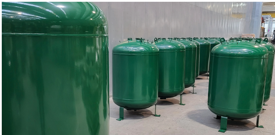
Underground tanks coated with PPG green epoxy powder coating at Antonio Merloni Pressure Vessels' plant in Matelica
