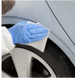
Ensure all swages and edges are abraded.
