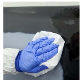
Clean the repaired area again before painting.
