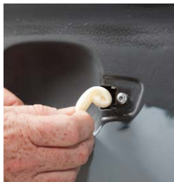
Ensure all swages and edges are abraded.
