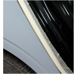
Thorough masking of apertures is essential.
