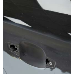
Clean the repaired area thoroughly before masking.
