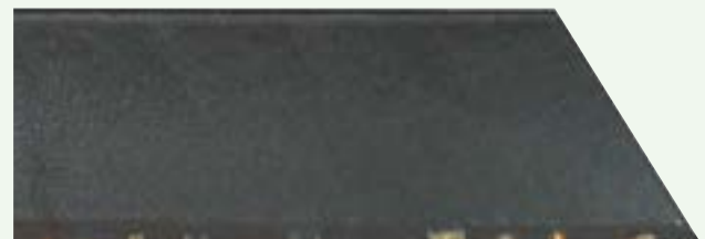
Conventional Electrocoat: >100 Rust Spots
