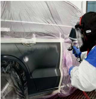
Apply a 100% first coat to DP5000 to the whole repair area.
