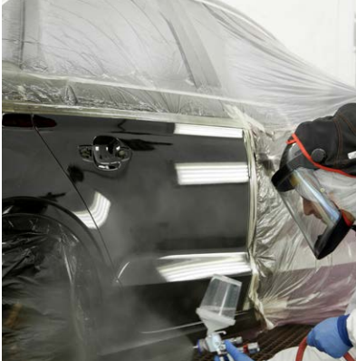
Inspect the final finish, allow overspray to clear the booth, then flash off for 5 minutes before initiating the recommended bake cycle.
