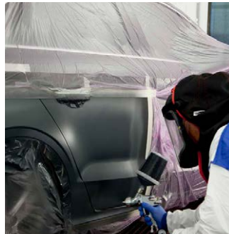
Apply a 100% second coat just inside the first.
