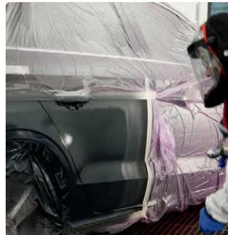
Apply a 100% third coat just inside the second coat.
