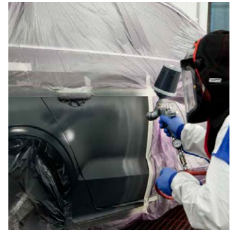
If needed a 100% fourth coat can be applied just inside the third coat
