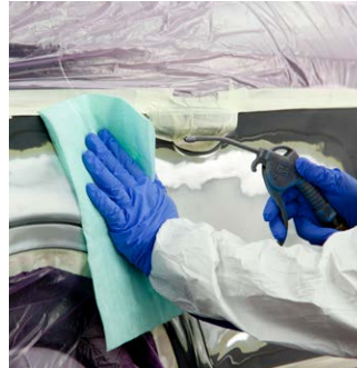
Blow off and tack the panel thoroughly.
