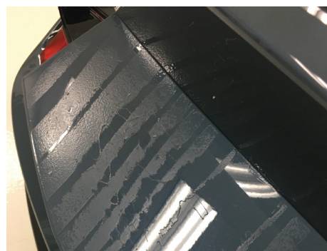
Previous vehicle wraps and adhesives should be removed
