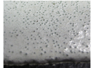
Material after heating with ideal 60% glass bead embedment for optimal performance
