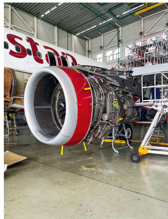
BELOW: Pratt & Whitney GTF engine issues have impacted the airline group considerably, with up to 13 A320neo Family aircraft grounded during the peak season in 2025 KEY-LEE CROSS
