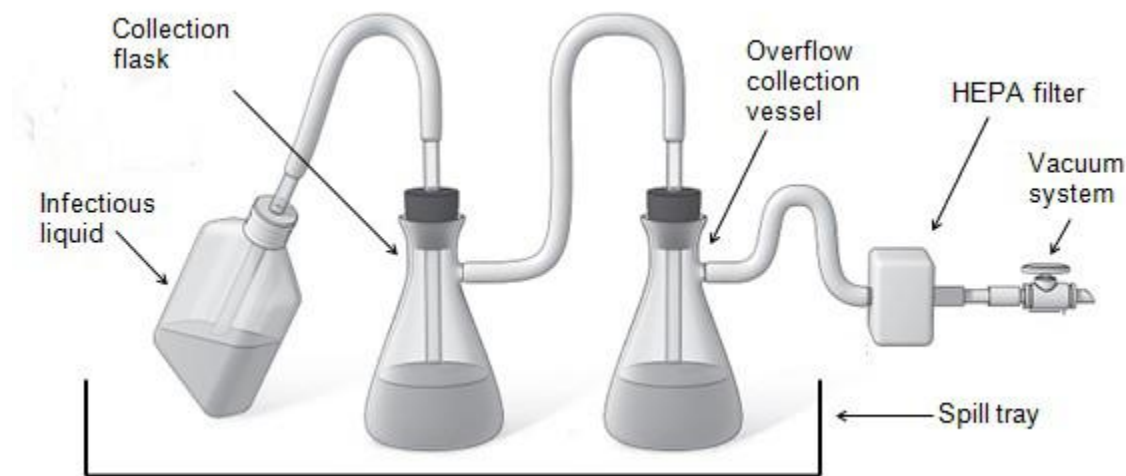
Figure 10-1: HEPA filtered overflow set to prevent microbiological contamination of vacuum systems.
