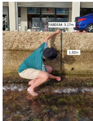
Figure 9 Photo of one of the elevation measurements in Kralendijk, illustrating the difference between the measured and the FABDEM elevation
