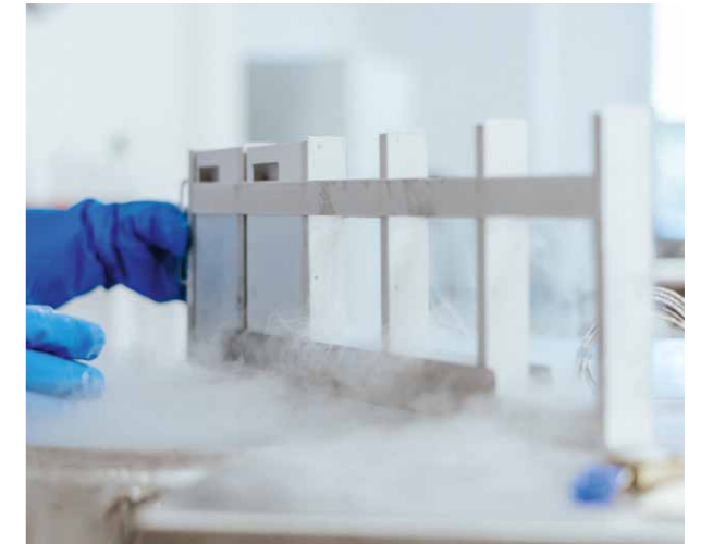
Thick vapour of nitrogen is released when the cryogenic tank is opened to put in the stem cells
