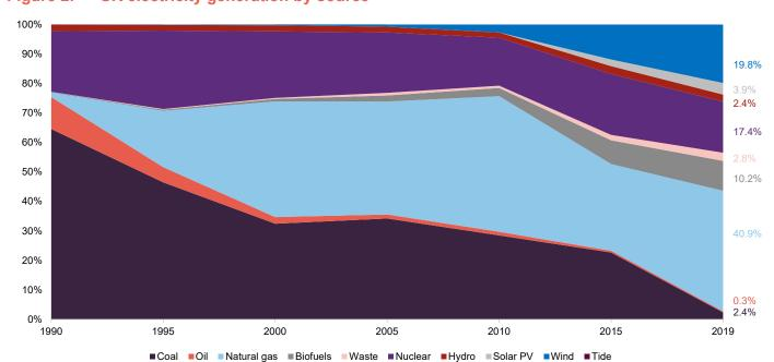
Figure 2: UK electricity generation by source
