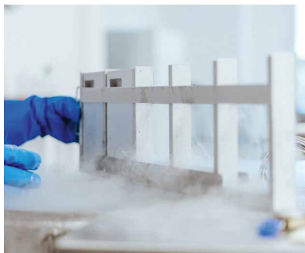
Thick vapor of nitrogen is released when the cryogenic tank is opened to put in the stem cells
