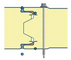
Side Lap Details (120, 150, 170, 200, 220 mm) - Visible fixing, triple joint,
