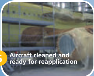
5 Topcoat removed by high pressure washing
