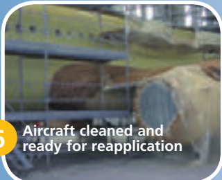
5 Topcoat removed by high pressure washing
