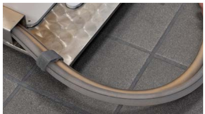
Proper hose routing
