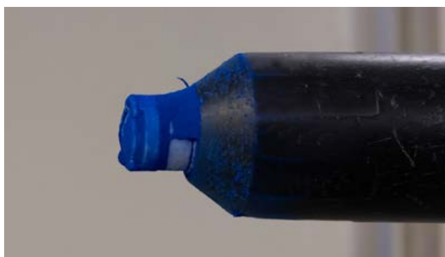
Build-up on the spray nozzle
