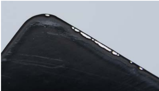
Powder coating is not adhering at the edges
