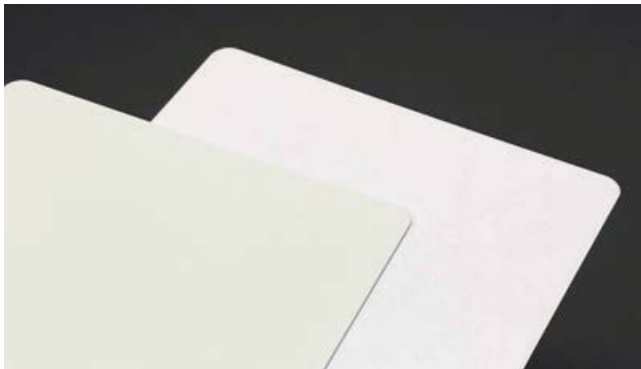
Yellowing due to overcuring
