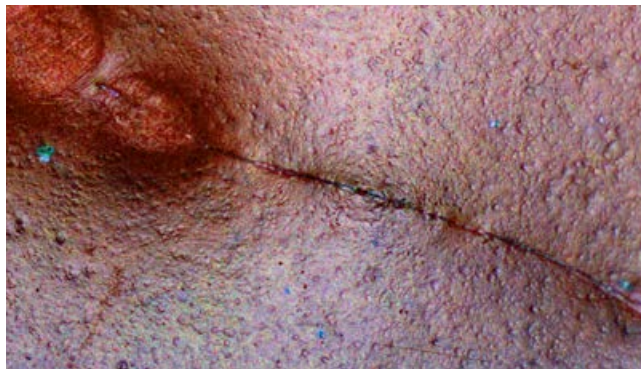
Contamination due to fibers (microscope)
