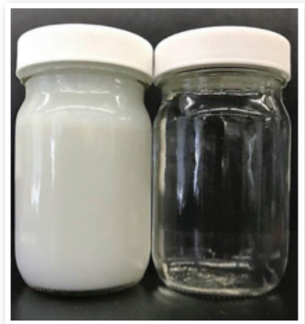
Figure 17 Comparison of Feed and Permeate Appearance
