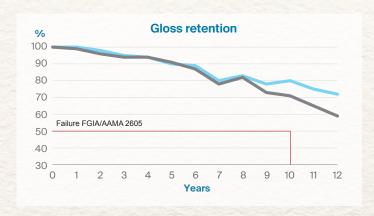
\*All tests performed by independent third-party laboratory using Section 8.9 of AAMA 2605 standards.
