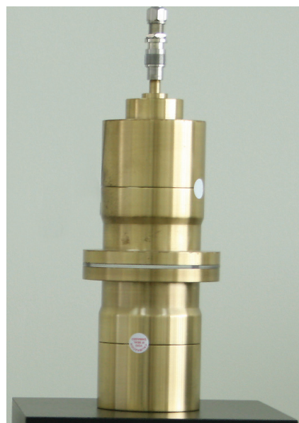
Fig 1. ASTM D4935-10 test fixture for SE measurements at f = 30 \text{ MHz} - 1.5 \text{ GHz} .
