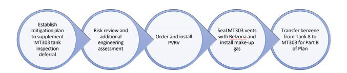
Available engineering shows Tank 8 cannot be sealed, which is why modelled emissions were projected to be elevated. Other emission reduction options could be considered with further/additional engineering.
