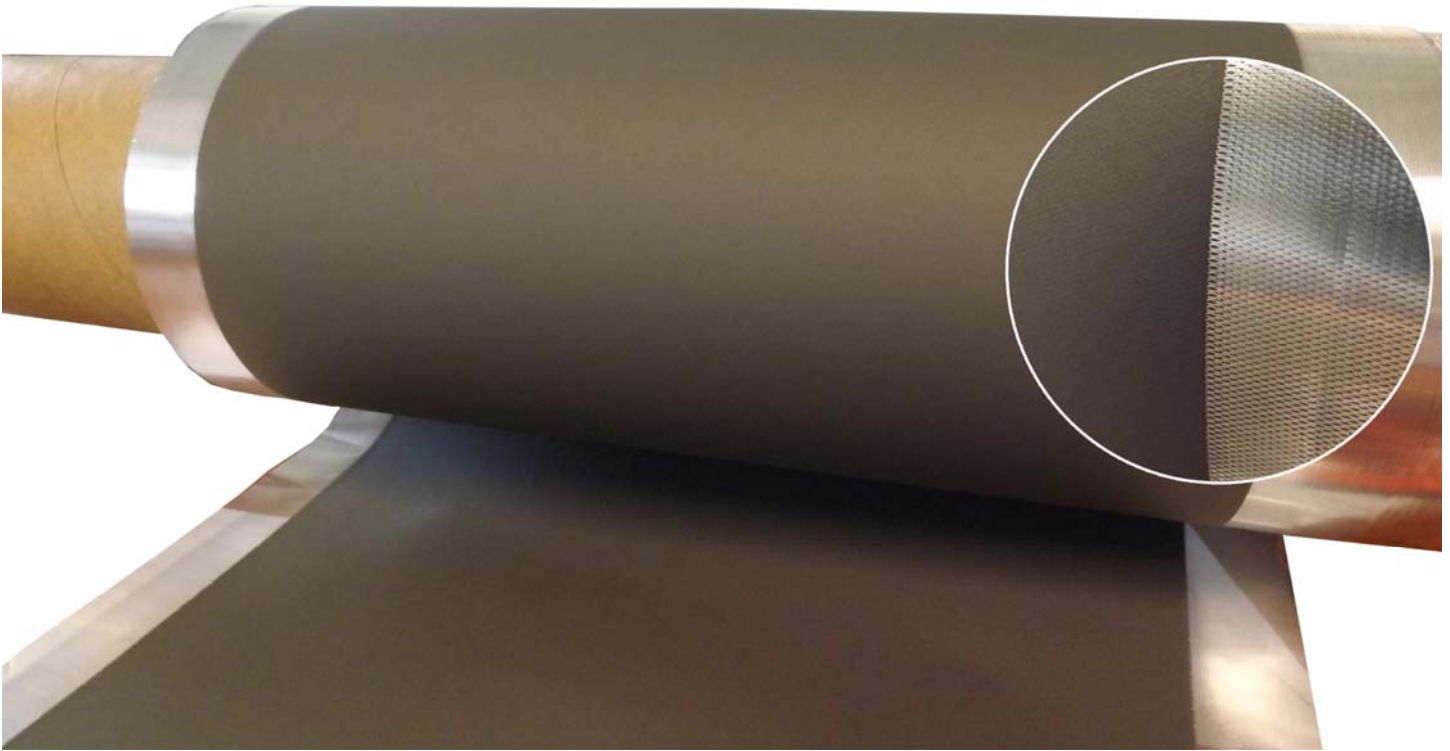
Double Sided Single Pass Coating using MEGTEC Coater with Vertical Injection
