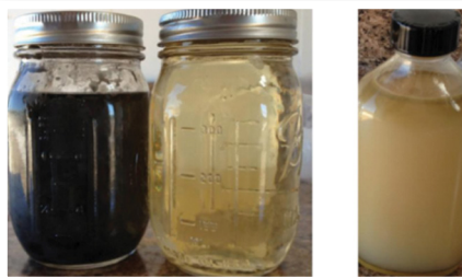
Figure 6 Oil-contaminated water and permeate following treatment (left) Oil-contaminated water after incumbent chemical treatment process (right)
