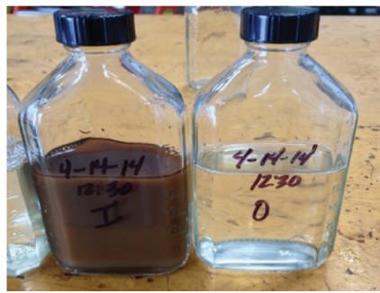
Figure 5 Oil flow-back water from a Middle East oil feed (left) Filtered permeate (right)
