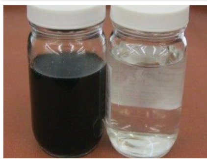
Figure 7 Produced water provided by major U.S. drilling company (left) Filtered permeate (right)
