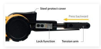
To release the belt, press the tension arm towards the steel protect cover to disengage the lock function. Open the protect cover by loosening the cover knob.
