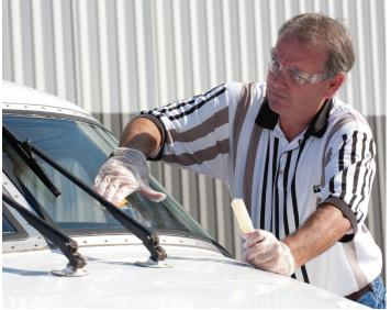
Surface Seal hydrophobic coating is an industry-leading rain/water shedding coating system designed for glass and anti-static coated glass windshields.
