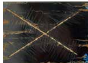
Conventional Ecoat CRS - 15' @ 175°C (347°F)
