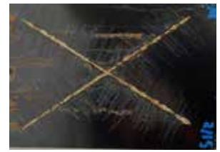
PPG POWERCRON® 10X™ CRS - 15' @ 150°C (302°F)
