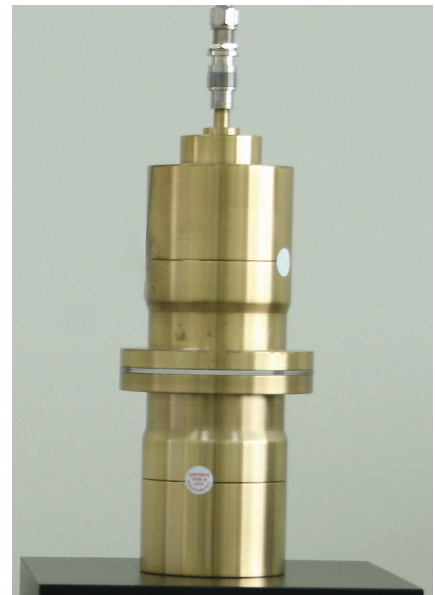
Fig 1. ASTM D4935-10 test fixture for SE measurements at f=30 Mhz - 1.5 Ghz.
